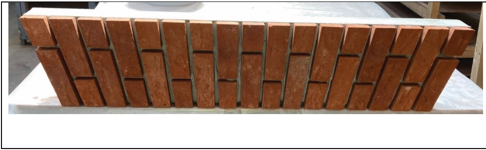
Figure 1 Lightweight Brick Clad Insulated Panel
